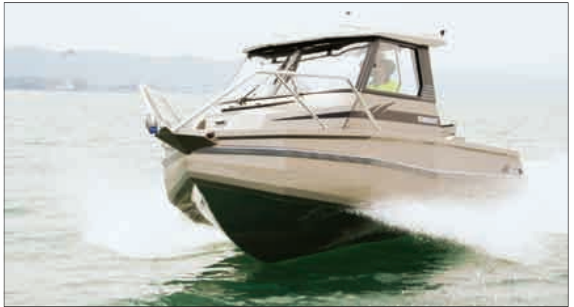
The Generation III hull pushing the spray downward and away.
