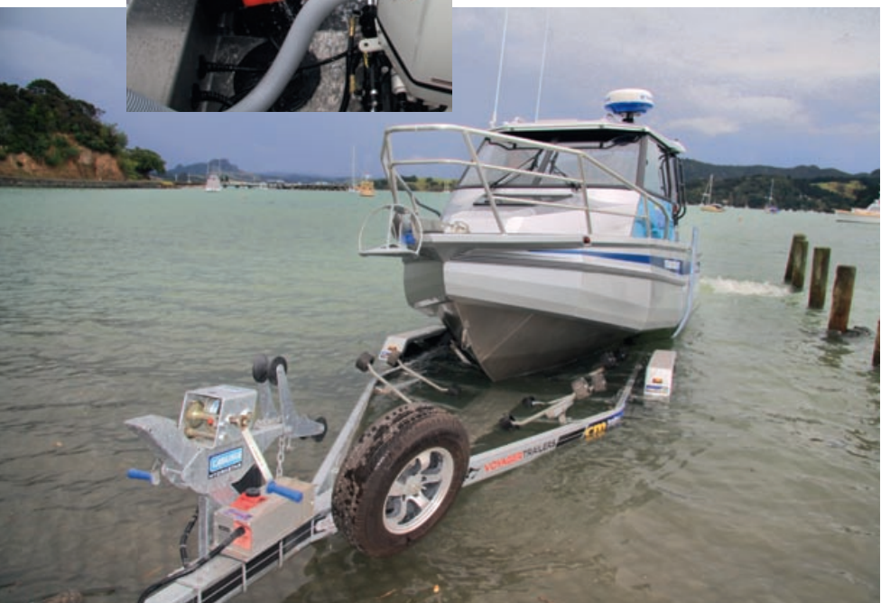
Below: guide poles help to position the boat on the highly spec'ed Voyager Elite trailer.
