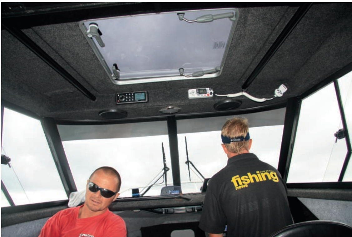
A side-opening roof hatch allows for good communication between the skipper and the spotter/cameraman on the roof.
