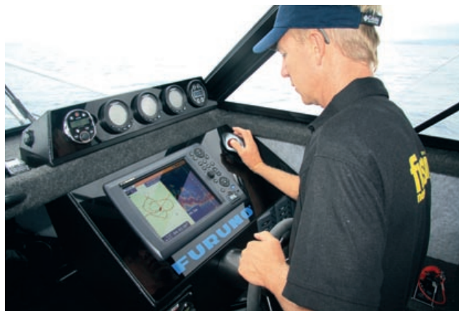
Left: at the heart of the helm station is the Furuno NavNet 3D which interfaces the sounder, chartplotter and radar functions. Right: Got 'Em On features great use of stowage space.
