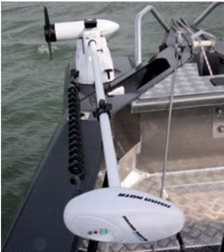
A bracket has been created to carry the MinnKota electric outboard.
