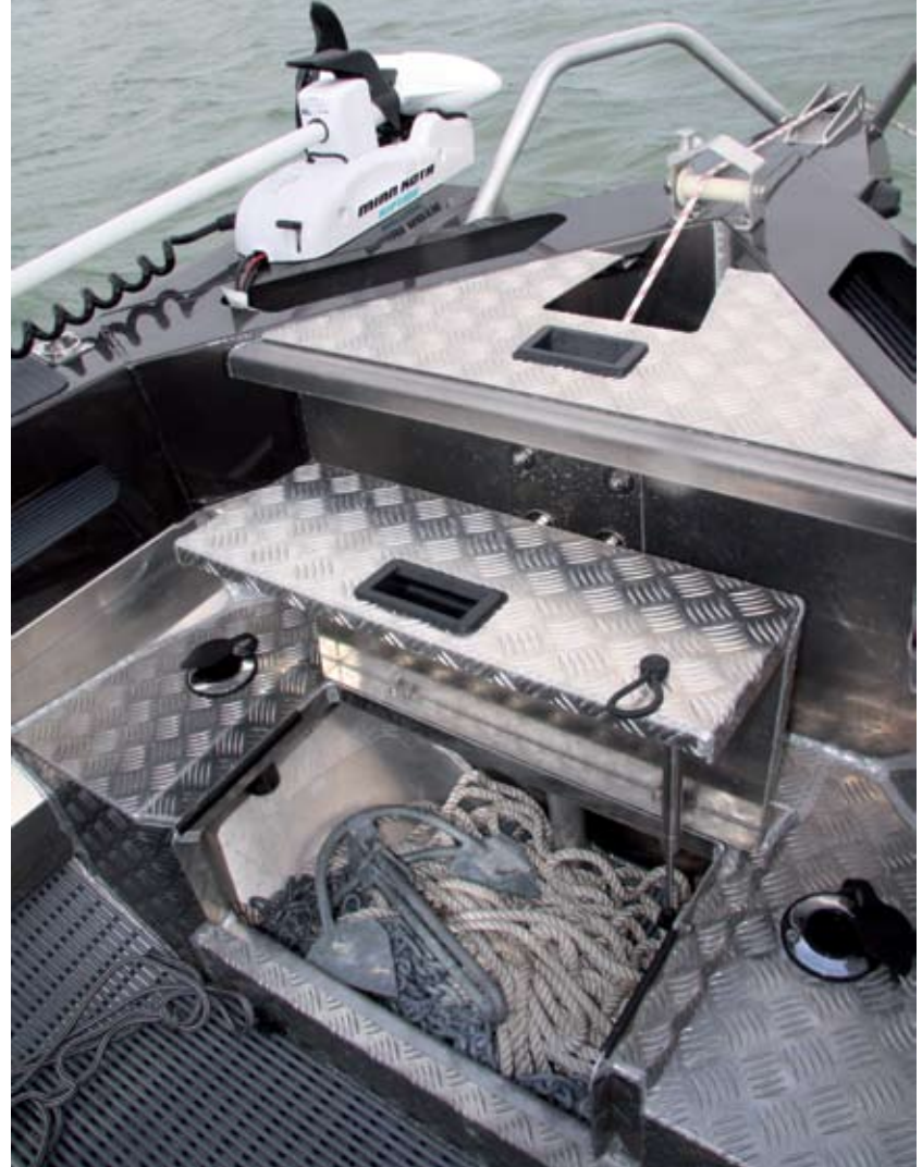
Beneath the forward casting platform is space for the spare anchor and the battery for the MinnKota electric motor.
