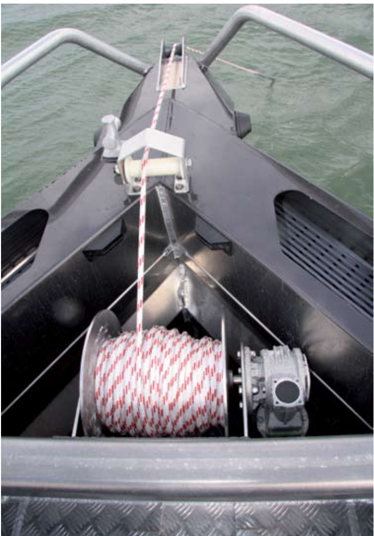
The Stress-Free system works well. A chequerplate cover fits over the top of the drum to protect it from the worst spray.
