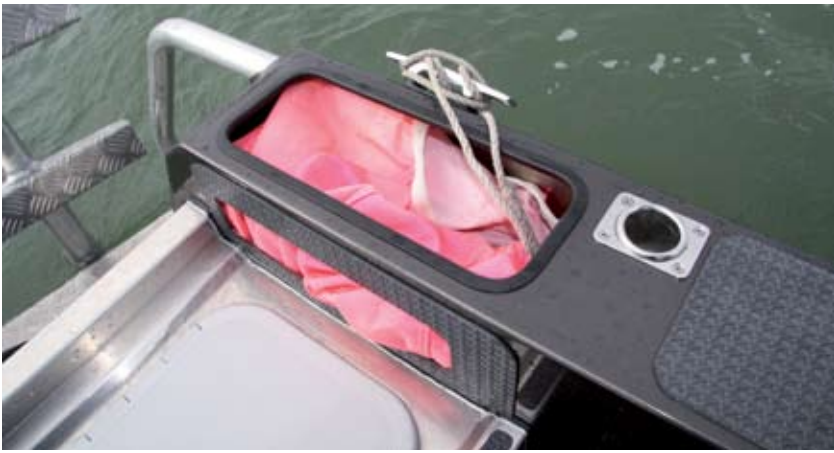
This compartment was designed specifically with the John Hewinson Canvas sea anchor in mind.
