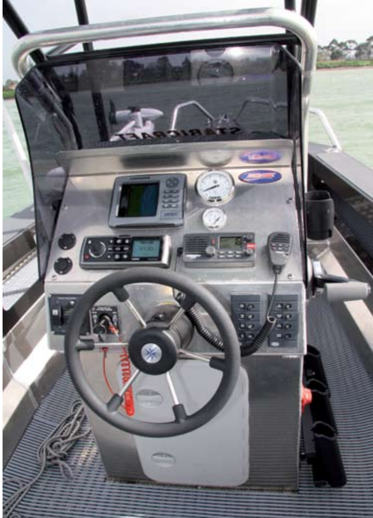
The centre console, incorporating the helm station with dry storage below the wheel.
